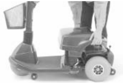
Figure 17. Rear Shroud Removal
